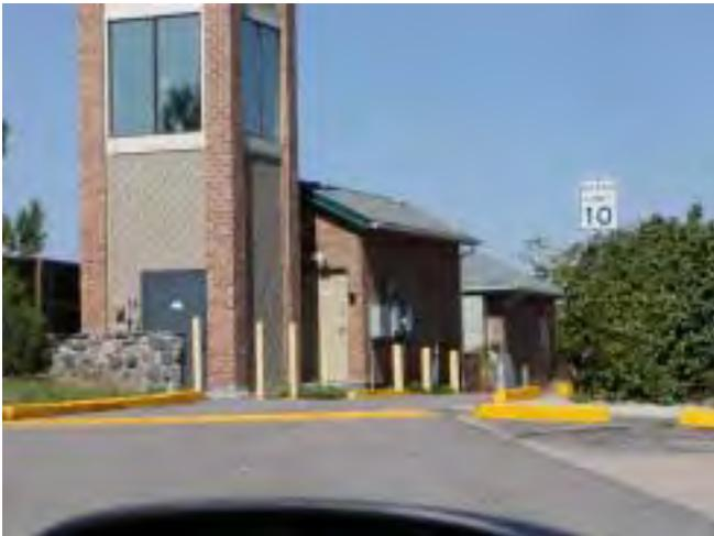
This design should qualify as meeting general design standards for “building mount” in industrial or large commercial areas, for example, but should not qualify as meeting HDS. Panels should be internal to the structure or appear elemental to the design. Accessory equipment structure is excellent because it completely conceals equipment and matches the surrounding context in architecture and scale.
